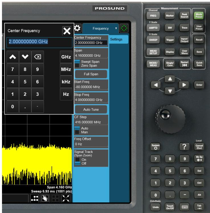
You can display the Numeric Entry Panel by touching any active function control while it is active, but you don't have to pop up the Numeric Entry Panel first, you can just start typing and it will pop up on its own, thus saving you a keystroke.
