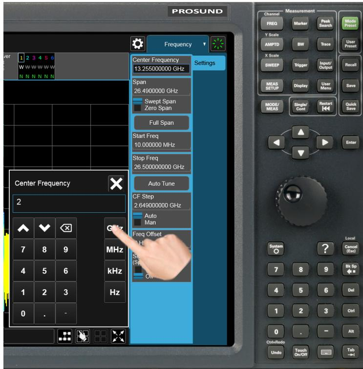
The Numeric Entry Panel disappears and, in the example, the active function value becomes 2 GHz.
