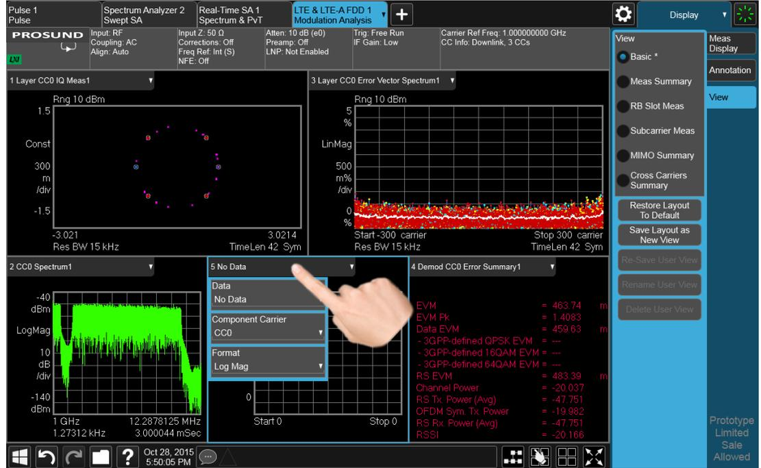
A panel drops down, containing a Data control for specifying window results. Some measurements, such as LTE-A in this example, also provide controls on this dropdown for specifying other window parameters, such as the Component Carrier and Data Format, Tap the Data control and you will see a list of available results for the window. In some cases, as in LTE-A, this will be a cascading list, due to the number of results available:
