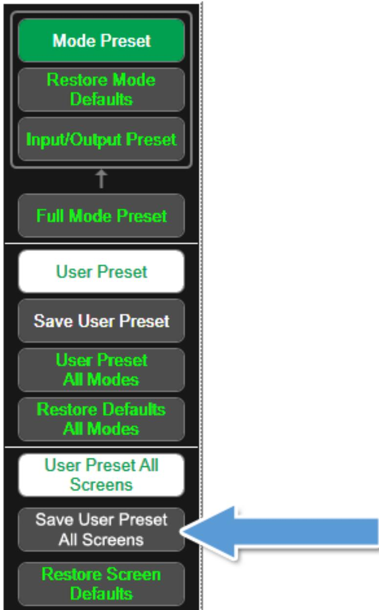
Besides the screen configuration, *all* of the Mode variables of all Screens are saved, including those reset by Mode Preset and those only reset by Restore Mode Defaults, as well as all of the Input/Output variables, so when you subsequently press the User Preset All Screens key, the instrument returns to the exact Screen setup that existed when you pressed the Save User Preset All Screens control.
