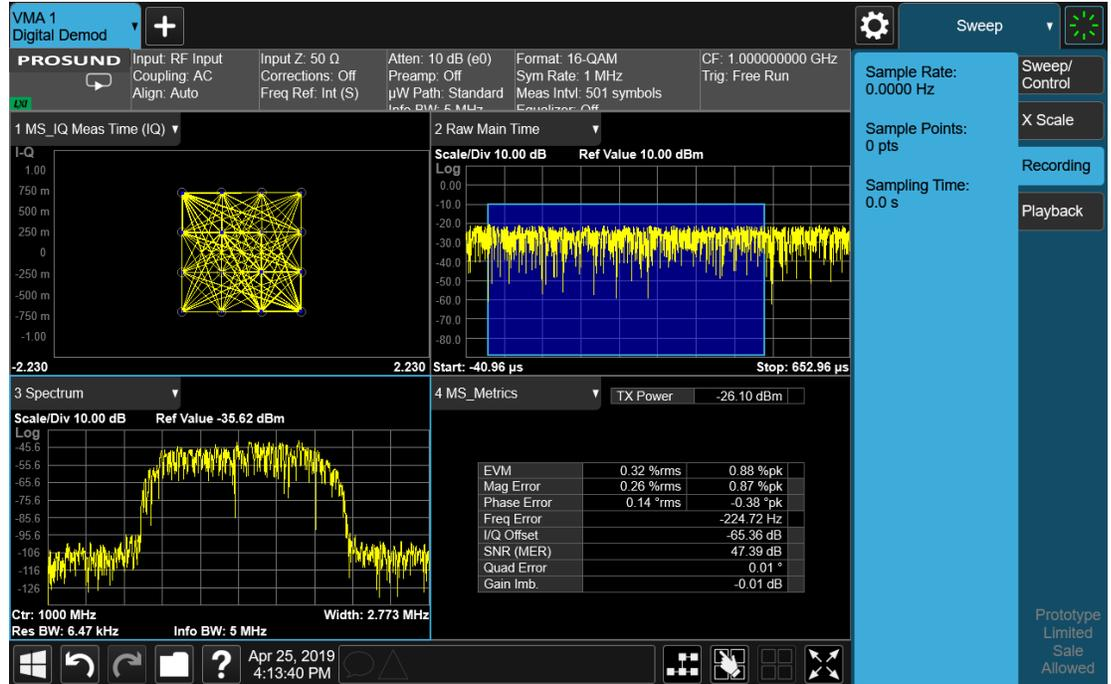
To save the data for the current measurement, press the **Save** hardkey (or the **Save** icon in the **File** panel) and press the **Recording** tab on the left side of the **Save** panel:
