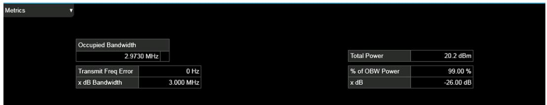
For the LTE-Advanced FDD/TDD and 5G NR modes, the metric result is shown as below:
